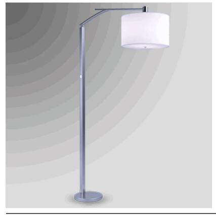
72" Matte Brushed Nickel Floor Lamp, "S" Arm with two medium base sockets, white on/off rocker switch on column at 48"AFF, 13' Silver fabric braided 45° cord, 16x16x10 White Linen HB Shade with top and bottom diffusers. (Ships as knock down)
